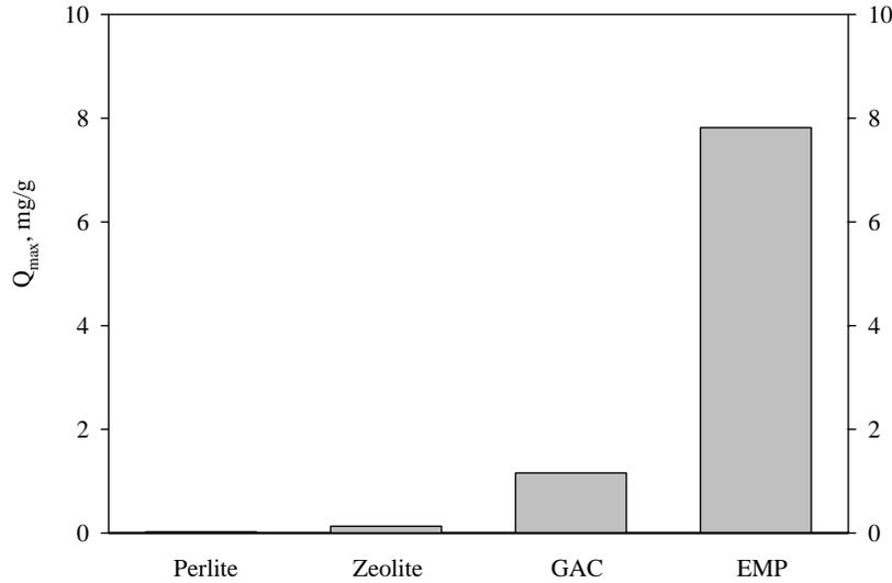
**Figure 3. Comparison of media maximum phosphate adsorption capacities by isotherms.**
