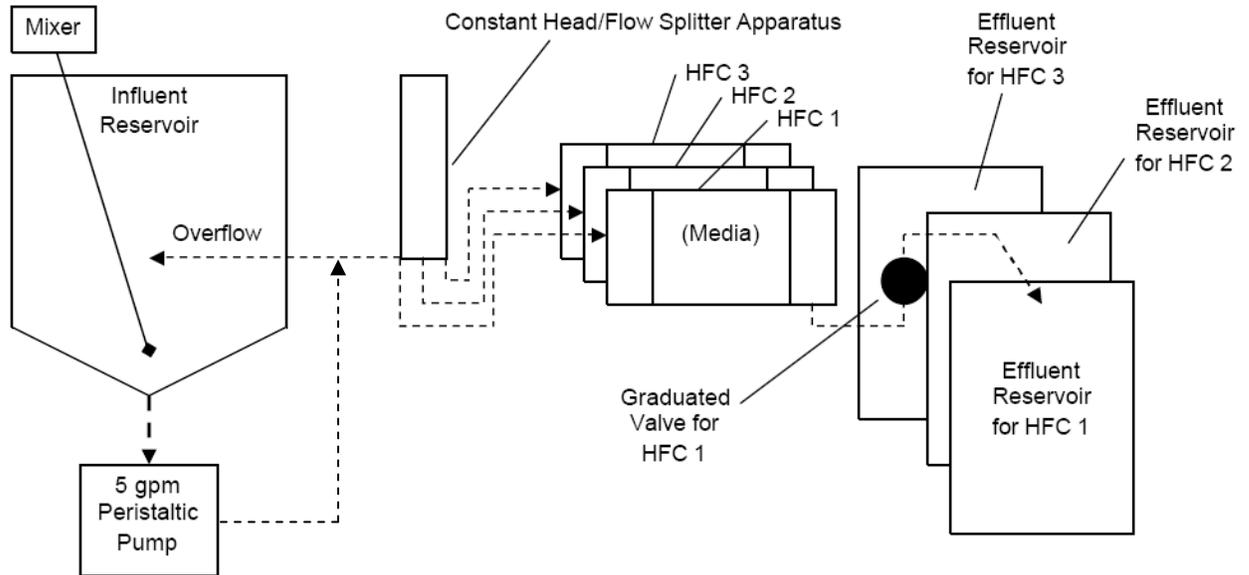
**Figure 1. Illustration of the testing apparatus for breakthrough experiment. Dashed lines represent flow. Graduated valves and effluent flow vectors for horizontal flow columns (HFC) of 2&3 have been left out for clarity.**
