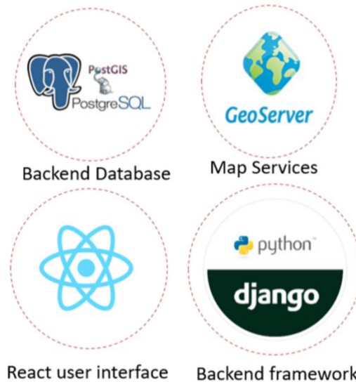
Figure B-1. Technology architecture of the SML Webtool, showing the integration of PostGIS for geospatial data storage, GeoServer for serving spatial data via web services (WMS/WFS), Django for backend processing and application programming interface (API) development, and React for frontend user interaction and visualization. The system is deployed with Amazon Web Services, Inc. to ensure scalability and secure cloud-based data access.
